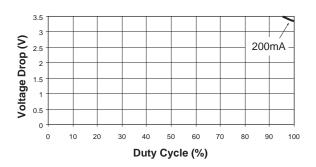
Device Duty Cycle vs. V<sub>DROP</sub> (V<sub>OUT</sub> = 2.5V @ 50°C)
